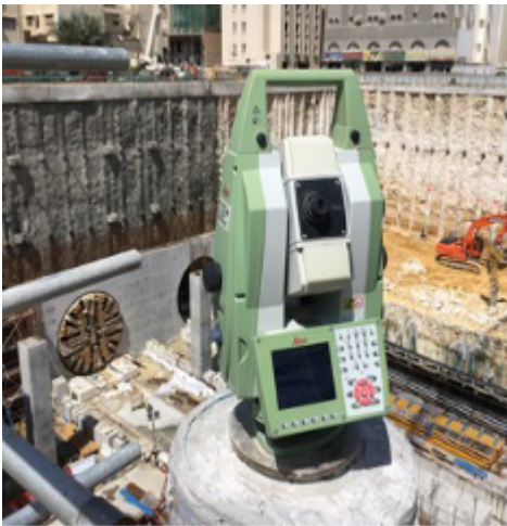
Automated motorized total station (AMTS) for tunnel 3D deformation monitoring
